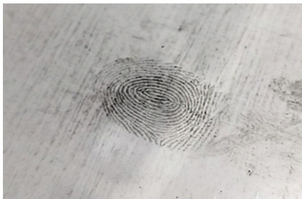
Figure 5: Development of latent fingerprint with the help of carbon powder on porous wooden surface
