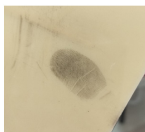
Figure 4: Development of latent fingerprint with the help of carbon powder on non- plastic sheet
